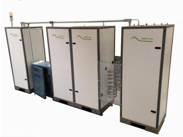
As 2 of the 3 catalyst vessels operate at temperatures well beyond what is typical for heated catalyst purifiers, ARM used Thermco furnaces and standard Thermco controls to maintain operating temperatures. Note the cooling coils between cabinet 2 and 3, theses were highlighted in the last newsletter (test data is presented in the article below).
