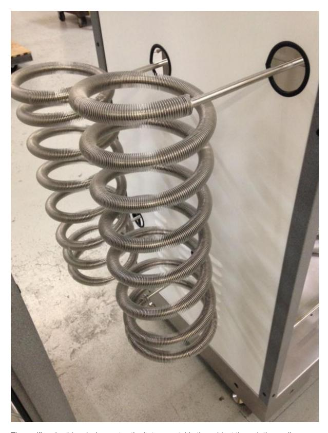
The purifier plumbing design routes the hot gas outside the cabinet through the cooling coils. One coil is plumbed between the second and third vessels and the other between the 3rd and 4th vessels.
